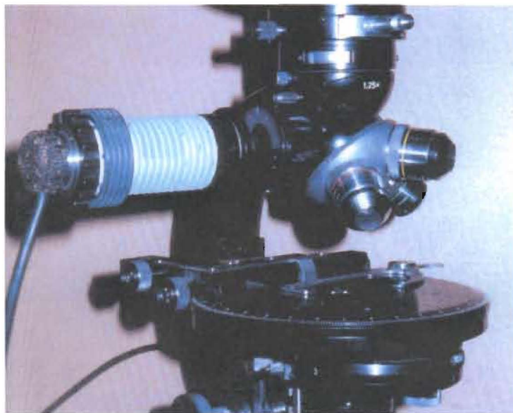
Fig.II: Objective Head Assembly for viewing opaque objects.
